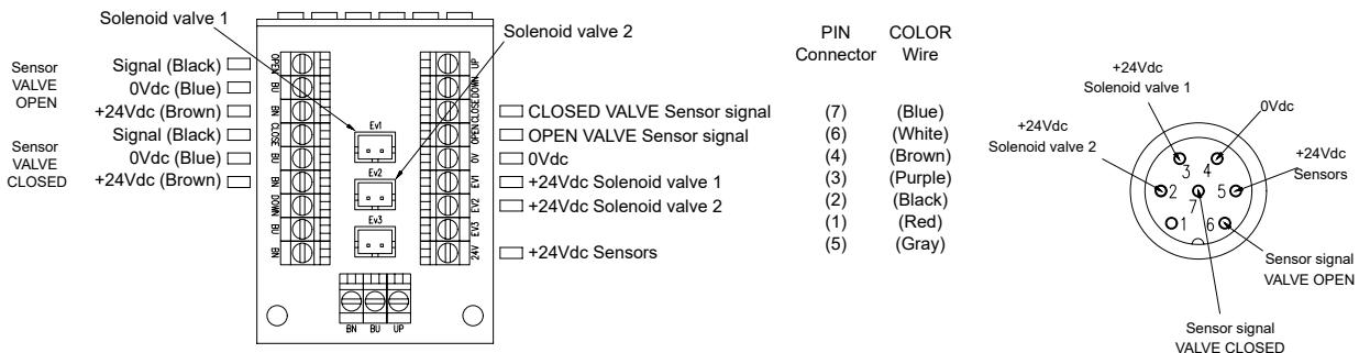
**1,2 PNP sensors with 2 solenoid valves (1 N.C. and 1 N.O.) for doble acting 7-pins connector**
