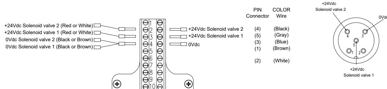
**2 microswitches with 1 solenoid valve normally closed and 5-poles wiring connection**
