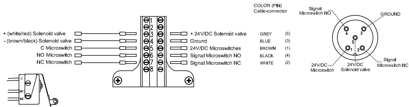
**2 microswitch with 1,2 solenoid valves normally closed and 7-poles wiring connection**
