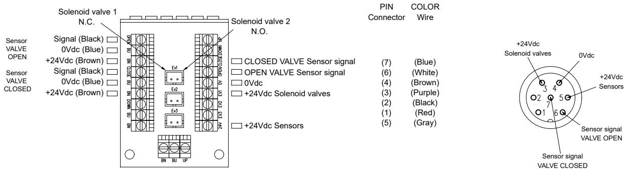
1,2 PNP sensors with 1 normally closed solenoid valves and 5-pins connector
