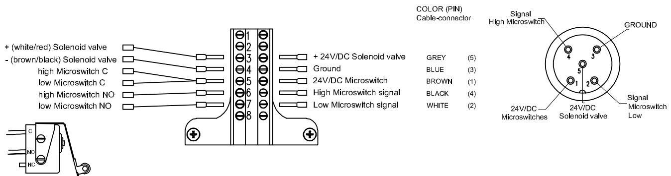
1 microswitch with 1 solenoid valve normally closed and 5-poles wiring connection
