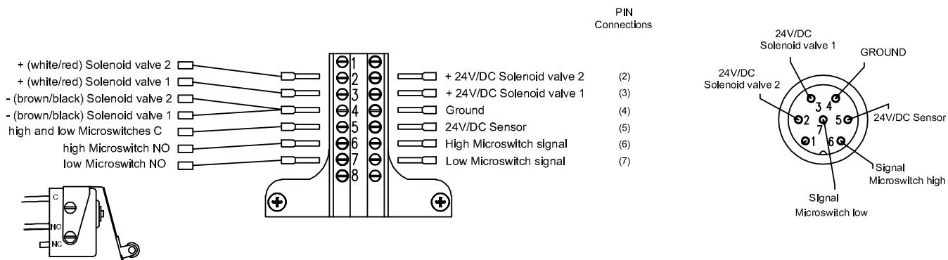
**1 microswitch with 1,2 solenoid valves normally closed and 7-poles wiring connection**
