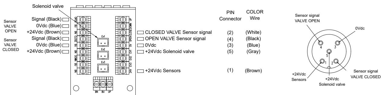
**1,2 PNP sensors with 2 solenoid valves (1 N.C. and 1 N.O.) for doble acting 5-pins connector**
