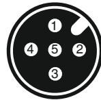
Five-pin M12 built-in socket, A-coded
