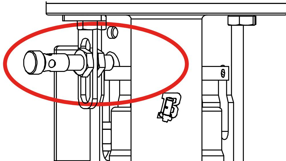
Close the valve and check that the sensor does not detect the cam as shown in the figure.
