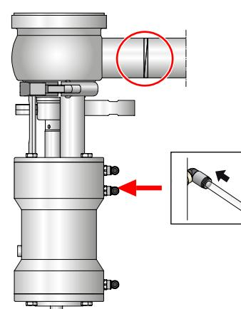
Weld it care/ try to make a stressless welding to avoid deformation on sealing areas. Check the valve for regular operation after welding. Only use pulsed arc welding and remember no gap between flange
