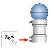
Adjust and regulate the proximity switch position until the lower middle section of the sensitive area is in correspondence with the upper edge of the upper shutter.
