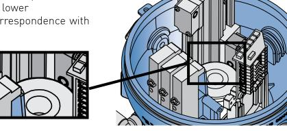
5 Activate the lower lift with regulated air at 6 bar in the upper air connection in the actuator.
