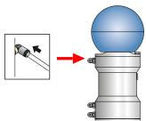
6 If the Proximity switch is correctly calibrated (screw positioning), it must NOT send a feedback signal, and its LED should be OFF. Lower seat is now consider open with the 1.59 mm downward movement offset set by the spacer.
