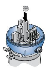
3 Screw the cam on the shaft, spacer will limit the lower lift downward stroke, when seat lift is actuated.
