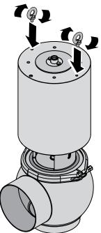
Once valve installation has been completed, remove the eyebolts and put the screws back in.
