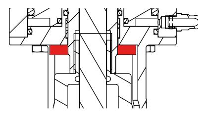
Execute upper valve lift and make sure the sensor switches status in the presence of the cam; if nothing happens, adjust the sensor.
