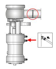
Weld it care/ try to make a stressless welding to avoid deformatin on sealing areas. Check the valve for regular operation after welding Only use pulsed arc welding and remember no gap between flange
