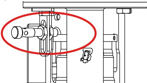
Close the valve and check that the sensor does not detect the cam as shown in the figure.
